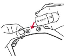
Press the R3 transmitter into the snaps of the chest belt.
