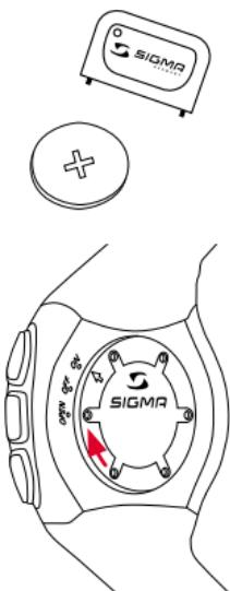
The battery CR2032 (Ref. No. 00342) is used in the running computer and battery CR2450 (Ref. No. 20316) in the R3 transmitter.
